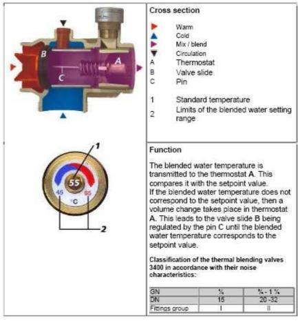
The warm water temperature has to be at least 5 K higher than the blended water temperature.
